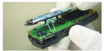
Now the UI module can be removed. Please take care of not to damage the board to board connector afterwards which is located on the CMT module.
