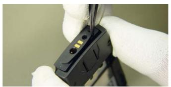
Turn around the B-Cover. If the System Connector is jammed, press with tweezers between cover and connector.
