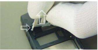
The second step is to push one hinge to the middle to lift up the Card Cover.
