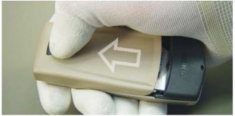
Push the unlock-button and move the battery cover to the System Connector direction.
