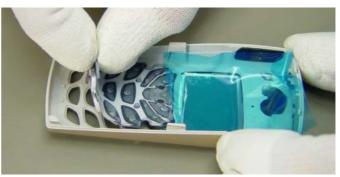
Remove the Keymat. It is always good to protect the window from the inner side.
