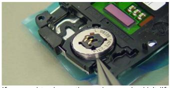
If you need to change the speaker you shouldn't lift it from the spring connectors. Take tweezers and lift the speaker as shown in the picture.
