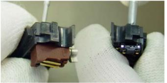
The System Connector contains Vibra Motor and Microphone, which can be easily pushed out from the System Connector.
