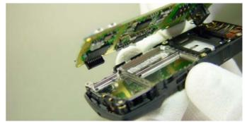
Lift up the CMT module LA5 carefully. Note that sometimes the battery connector gets stuck at the SIM Card Cover. Take care of not to bend the spring contacts of the battery connector.
